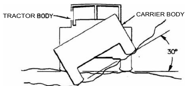
CARRIER BODY ROLL (LEFT OR RIGHT) \pm 30^\circ WITH RELATION TO THE TRACTOR BODY.
