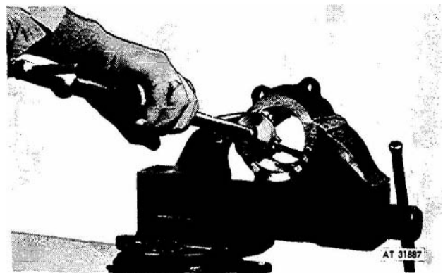
Figure 3-91. Removing bearing cup from housing.
