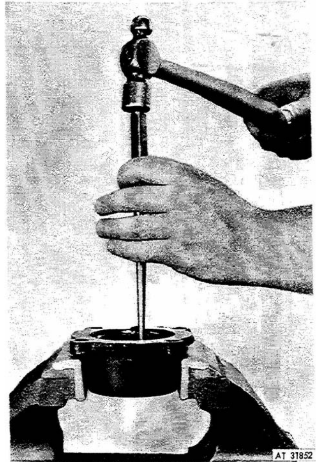
Figure 3-56. Removing input shaft oil seal.
